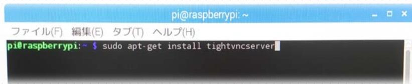
A screenshot of a terminal window on a Raspberry Pi. The window title is 'pi@raspberrypi: ~'. The menu bar shows 'ファイル(F) 編集(E) タブ(T) ヘルプ(H)'. The terminal prompt is 'pi@raspberrypi:~\$' and the command 'sudo apt-get install tightvncserver' is being typed.
